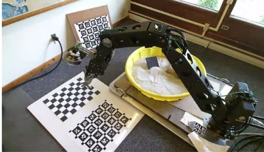
Figure 8: Testbed setup - a 6 degree-of-freedom hydraulic Kraft manipulator arm with a calibrated wrist-mounted fisheye camera and Apriltag fiducials on the base and in the environment
