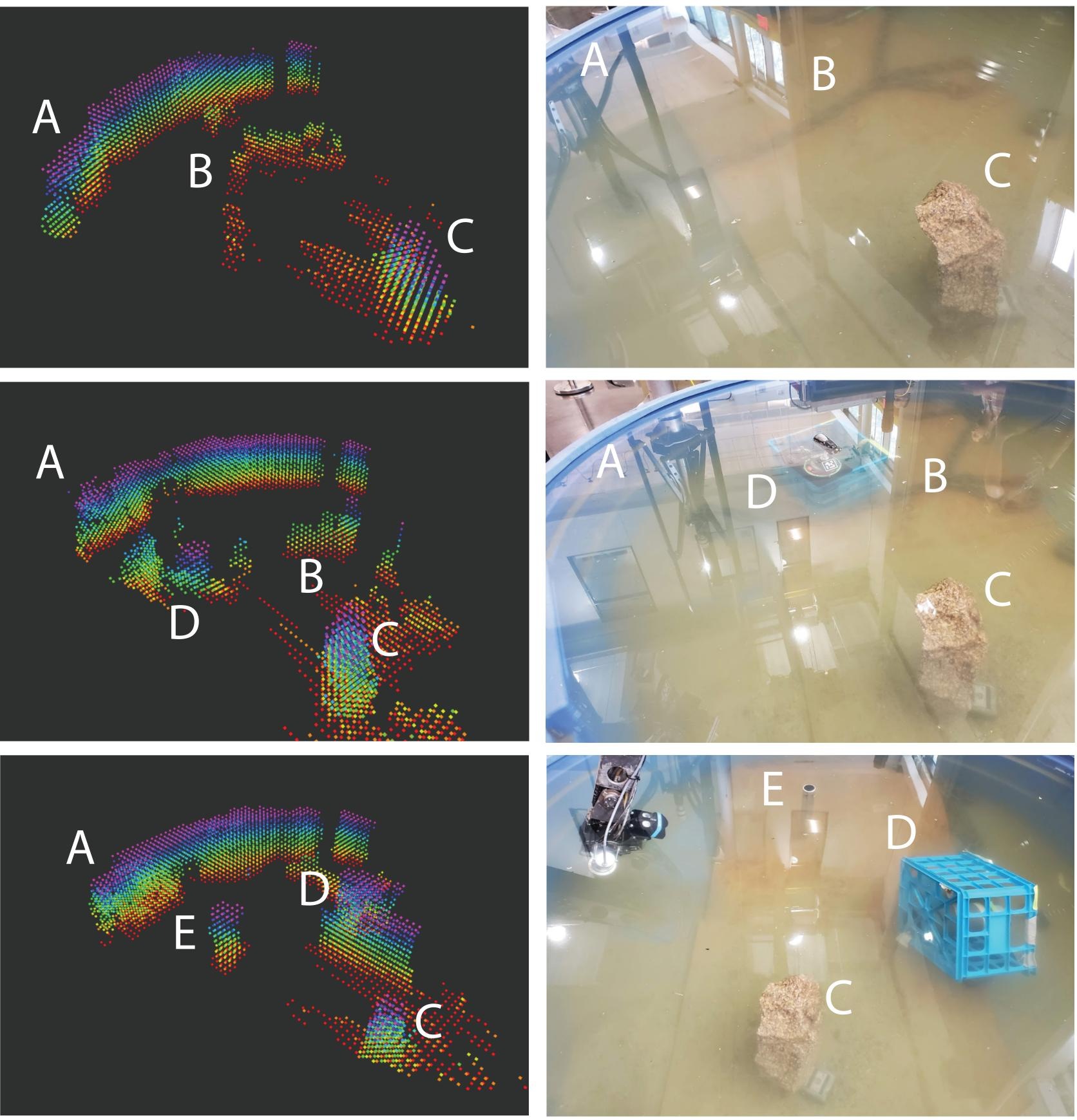
Fig. 3: (A) Tank walls, (B) chain, (C) rock, (D) tool crate, and (E) metal pipe are recognizable in the reconstructed data
