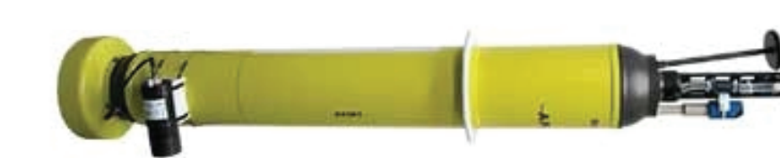
Fig 3: As of July 2020, 387 BGC Argo floats are used globally to take automated profiles of a variety of variables, including chlorophyll-a (Image source: http://www.teledynemarine.com/apex-biogeochem?BrandID=23 )
